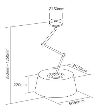
All hoods to be installed min. 700mm from hob, providing hob output does not exceed 11kW
