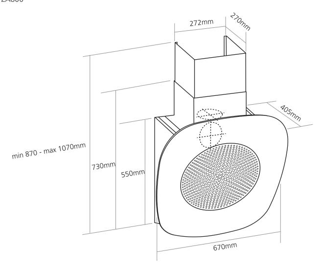
Between the lowest point of the hood and the hob the distance required is 450mm.
