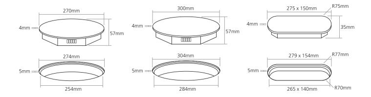
Space should be allocated underneath the work surface for the hob control box 270mm x 210m x 48mm. A minimum gap of 20mm is required beneath the hob fans and a 4mm gap must be left under the work surface at the front of the hob for ventilation
