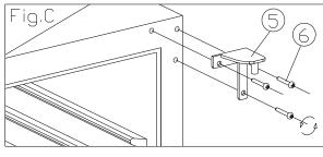
4. Rotate door at 180 degrees, assemble the door as per the per the above instructions, but in reverse.
