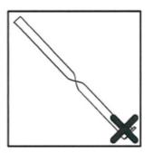
Trim the silicone hose to the right length for the installation. It must not be pulled taught, too slack leading to a 'U' bend or twisted. Please make sure the tube isn't pinched between the threaded stud and the braided hose as this may cause flow restriction. If the silicone is not installed correctly it may effect the performance of the system.
