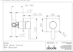
• Product mounted where: Wall • Recommended hole size: 60x60 mm
