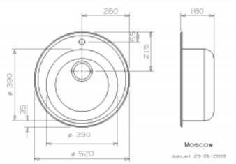
Tolerantie buitermaab per zijde 20.5mm Toleranz Aussenwage pro Beite 20.5mm Per side the outside tolerance negare 20.5mm
