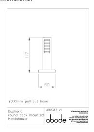
• Overall Height / projection: 117 mm • Exit reach: 65 - 1500 apx. mm
