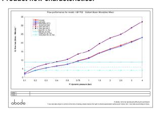
Min / Max water pressure: 0.2 / 5.5 bar
