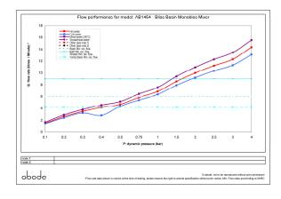
Min / Max water pressure: 0.75 / 5.5 bar
