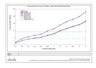
• Min / Max water pressure: 0.3 / 5.5 bar • Part G mixed flow rate at 3 bar (I/m): 19.83
