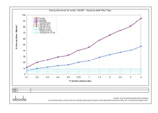
Min / Max water pressure: 0.1 / 5.5 bar
