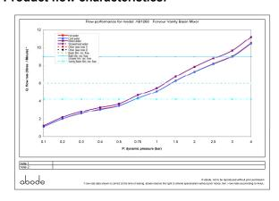
• Min / Max water pressure: 0.75 / 5.5 bar • Part G mixed flow rate at 3 bar (I/m): 9.68
