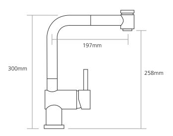
Note: Pull out hose extends by 460mm Worktop cut-out 35mm required
