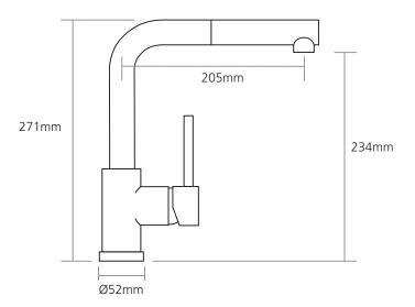
Note: Pull out hose extends by 660mm Worktop cut-out 35mm required
